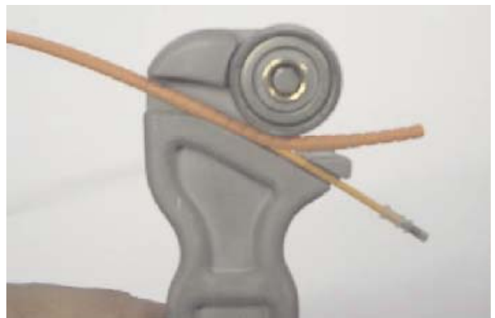
Figure 5: Tube cut and ready to be removed.
