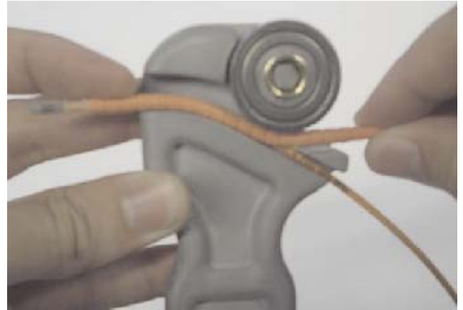
Figure 3: OFPT pulled to cover more of the cable.
