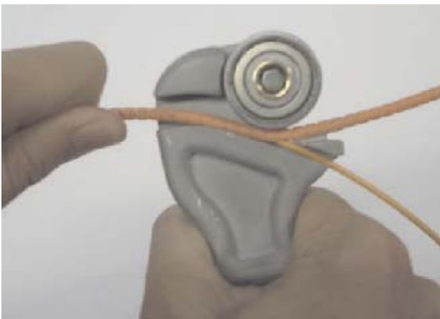
Figure 4: Remaining cable and OFPT pulled through.
