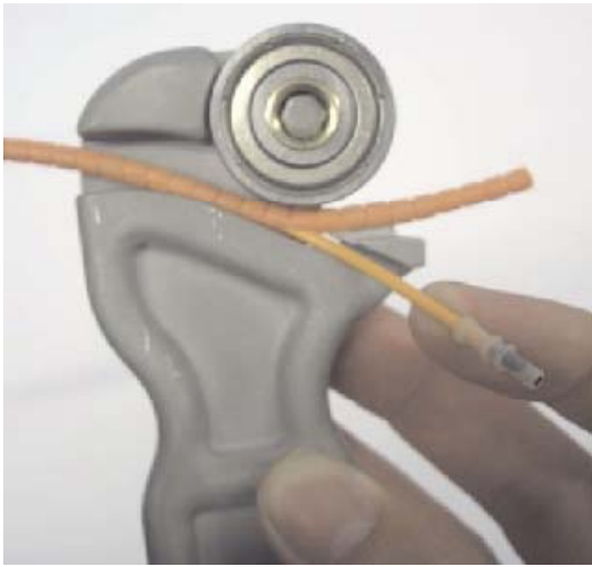
Figure 6: Pushing home the remaining section of OFPT.
